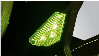
Buddy Light System LED color changes instantly show remaining air status and help locate the wearer in low visibility Green: Normal Operation / Red: Low Pressure Warning / Yellow: Low Battery
