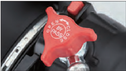
By-pass Valve Emergency escape valve for direct air supply to the facepiece in the event of demand valve failure
