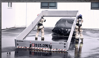
Covering the burning vehicle with an immersion tank
