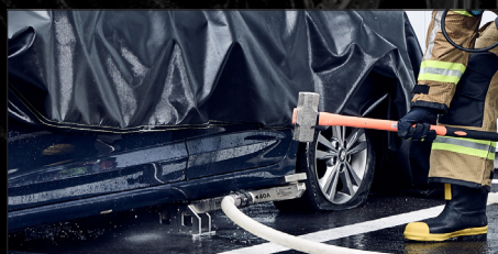
5. Penetrate with a hammer
