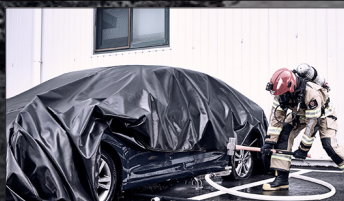
Piercing the lower battery with Seesaw and injecting fire extinguishing water
